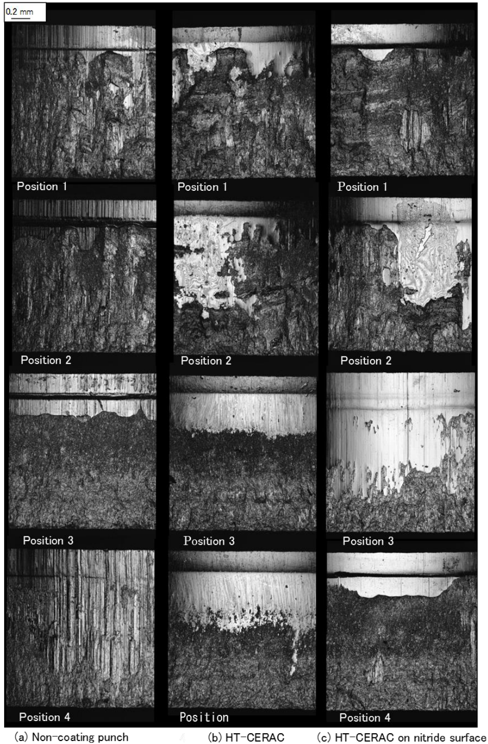
Fig. 4. Pierced surface observed by microscope.
