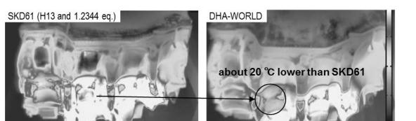
Figure 3 Comparison of the temperature profiles on the upper slide cores at 2 minutes after die opening.
