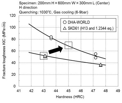
Figure 5 Fracture toughness
