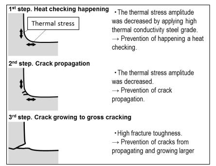
Figure 4 Schematic diagram of the gross crack mechanism. (Comments: The advantages of DHA-WORLD compared with SKD61)
