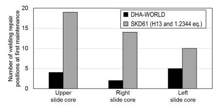
Figure 1 Number of welding repair positions at the first maintenance.
