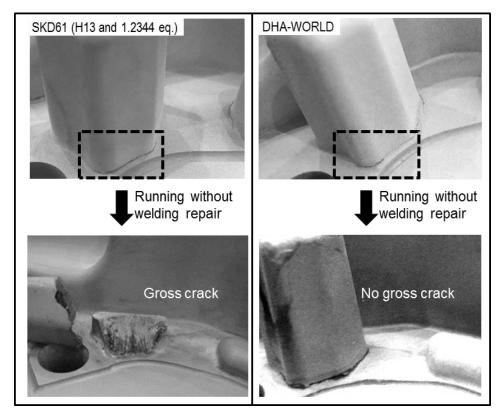
Figure 2 Comparison of the die appearance photographs at the gross crack positions.
