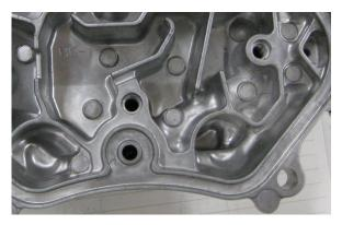
Figure 9 A part of Al die cast product where internal soundness was improved by the application of DHA-THERMO core pins.
