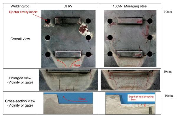
Fig. 9 Heat checking test result by actual die casting machine.
