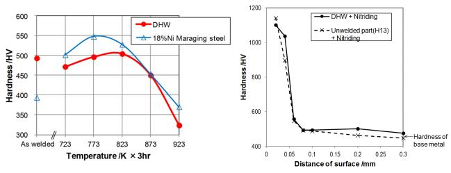
Fig. 10 Hardness with post-heating.
