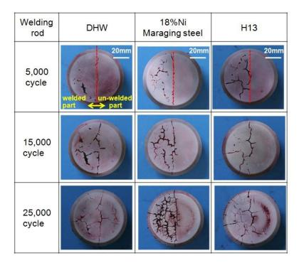
Fig. 8 Heat checking observed on the test specimens.
