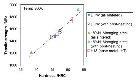
Fig. 19 Tensile strength at room temperature.
