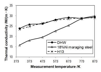
Fig. 6 Thermal conductivity of the part as welded.
