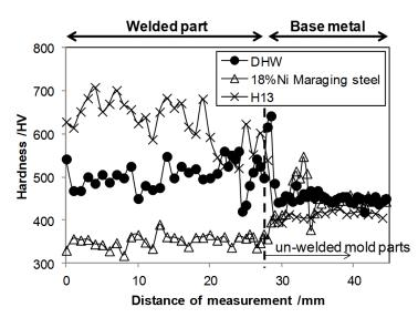
Fig. 4 Hardness distribution as welded.
