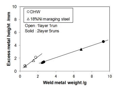
Fig. 12 Relationship between excess metal height and weld metal weight.
