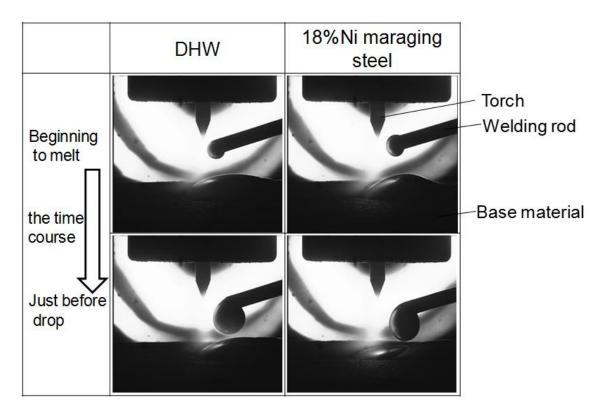
Fig. 13 An example of shots showing the behavior of droplets.
