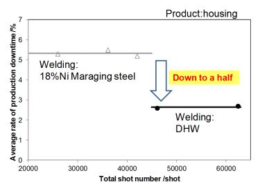
Fig. 15 An example of the application of DHW: reduced down time.
