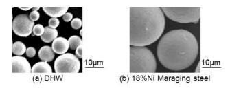
Fig. 16 SEM observation of powders used for laser sintering.
