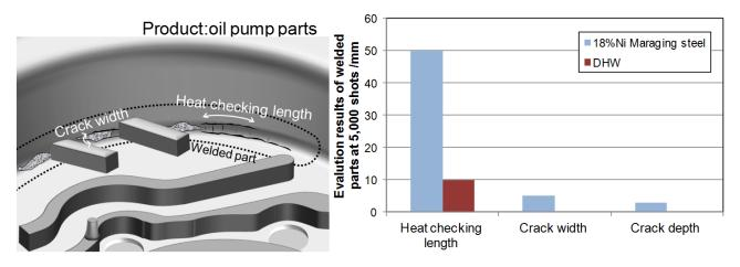
Fig. 14 An example of the application of DHW: Superior heat checking resistance.
