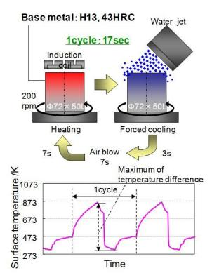
Fig. 7 Heat checking test procedures.
