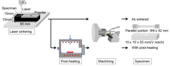
Fig. 17 Sampling procedures of tensile specimens.
