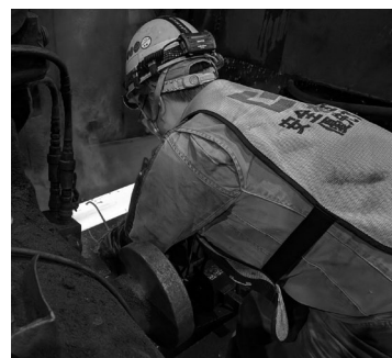
Fig. 1 Manual measurement using calipers on hot steel.
