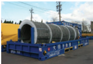
Special uncovered containers for steel materials that can be loaded on both trains and trailers
