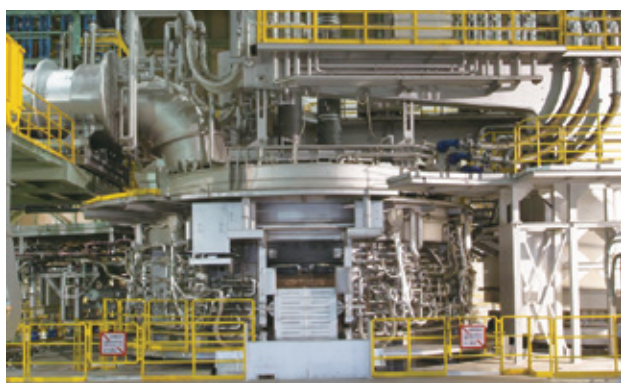
Energy-saving electric furnace with a rotation drive
