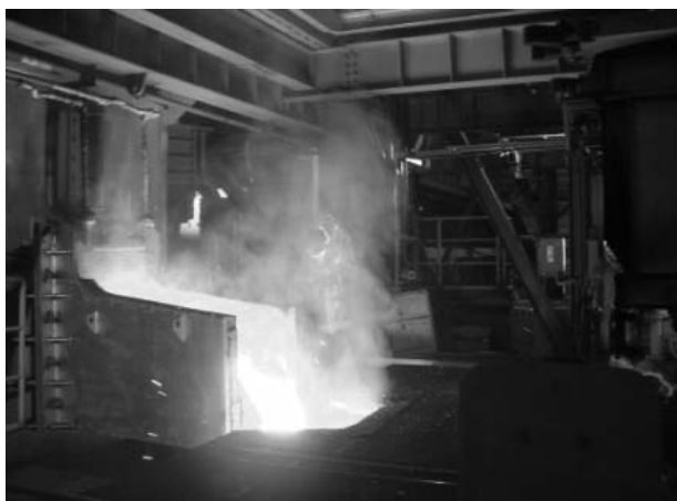
Fig.2. Metal tapping at SAF of Inmetco process.
