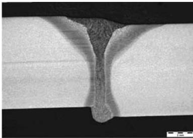
Fig. 4. Cross-section through hybrid weld made over joint with 0.8 mm of mismatch, focusing laser 2 mm below top of root face.
