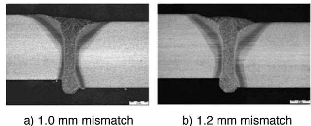
Fig. 6. Cross-section through adaptively controlled hybrid weld made over joint with hi-lo mismatch of 1.0 mm a) and 1.2 mm b).
