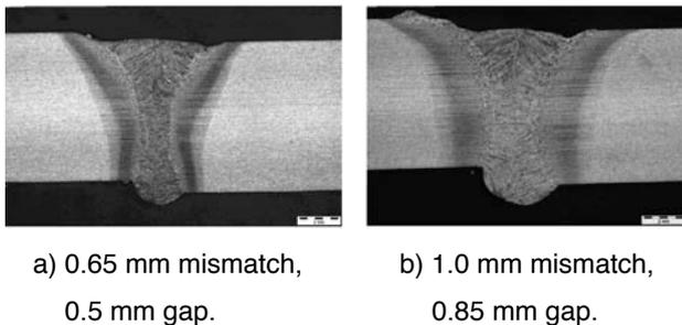
Fig. 8. Cross-sections through adaptively controlled hybrid weld made over joint with both mismatch and gap.
