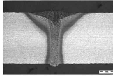
Fig. 2. Cross-section through hybrid weld made over flush, close fitting V butt joint. 2 mm scale bar.
