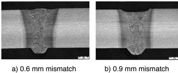
Fig. 7. Cross-sections through adaptively controlled hybrid weld made over joint with gap of 0.6 mm a) and 0.9 mm b).
