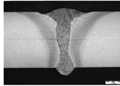
Fig. 5. Cross-section through hybrid weld made over joint with 0.5 mm wide gap, welding at 1.2 m/min with wire feed rate of 9 m/min.
