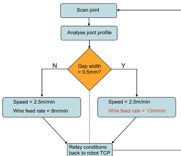
Fig. 1. Example of adaptive control algorithm.
