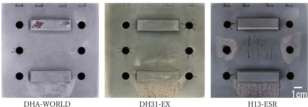
Figure 8 Heat checking test result: The appearance of test specimens after 10,000 shots.
