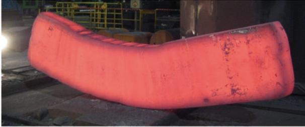
Fig. 1. Bent ITER parts by forging.
