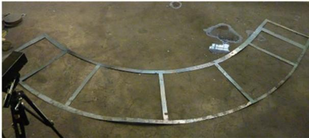
Fig. 2. Example of the gabari (gauge template).
