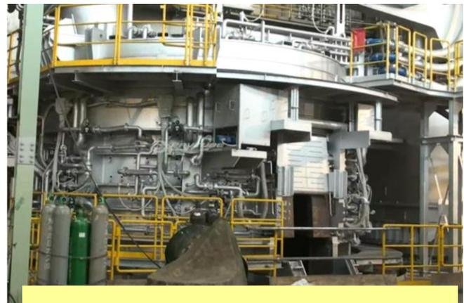
**STARQ (Arc furnace with a rotation drive)**
