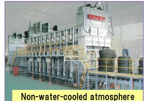
Non-water-cooled atmosphere heat treatment furnace
