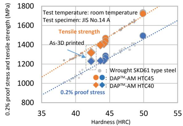
Fig. 3. Relationship between hardness, 0.2% proof stress, and tensile strength of DAP™-AM HTC<sup>3</sup>.
