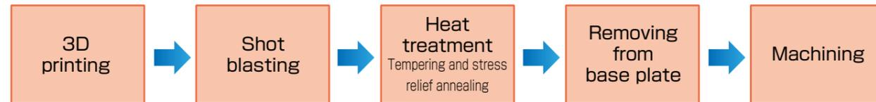
Fig. 11 Typical mold manufacturing process using DAP™-AM HTC.
