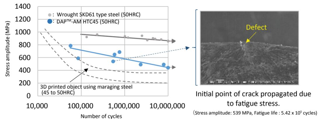
Fig. 5 Fatigue strength and typical fatigue fracture surface of DAP™-AM HTC<sup>3</sup>.
