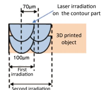
Fig. 9 Image of laser irradiation (2 times) to form the contour part.
