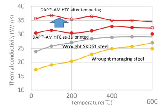
Fig. 2 Comparison of thermal conductivity. (Laser flash method)
