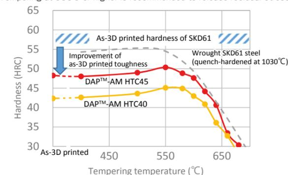
Fig. 1 Correlation of the hardness between as-3D printed and tempered after 3D printing. (Tempering [T°C × 1h] 2 times, base plate temperature 200°C)
