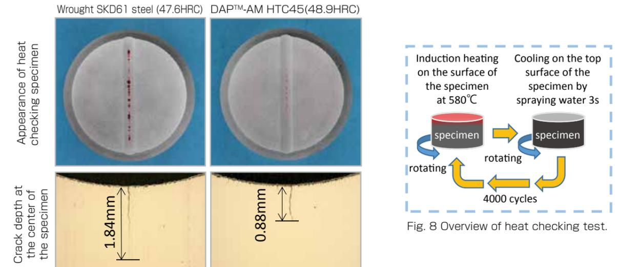
Fig. 7 Heat checking test results<sup>3</sup>. (Notch shape: R=6mm, depth 1mm)
