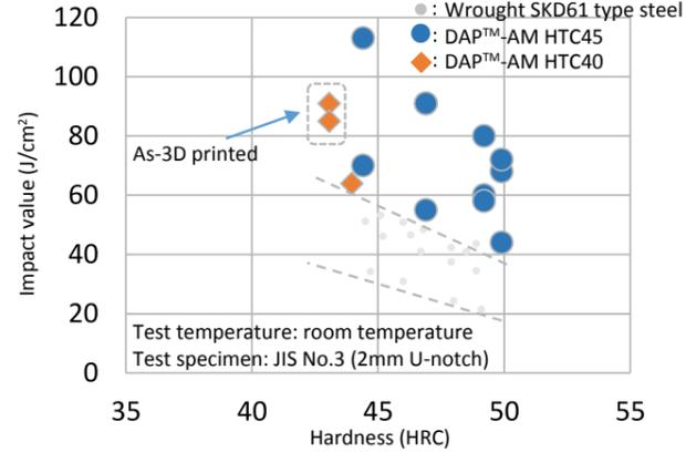
Fig. 4 Relationship between hardness and impact value of DAP™-AM HTC<sup>3</sup>.
