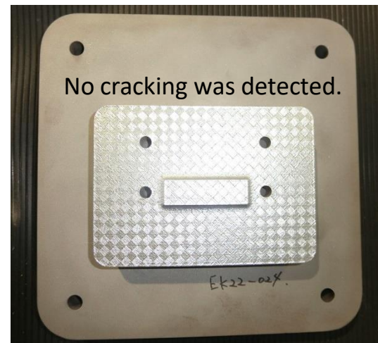
Fig. 4 Appearance of the 3D-printed test mold
