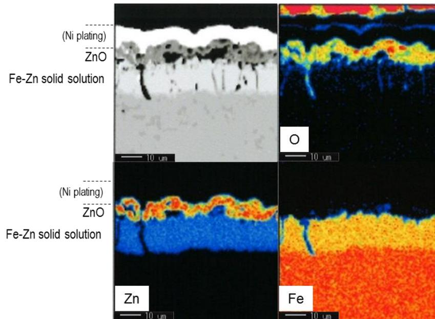
Fig. 2 EPMA analysis near surface of steel sheet after heating.
