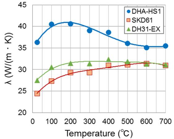
Fig. 6 Thermal conductivity of DHA-HS1.
