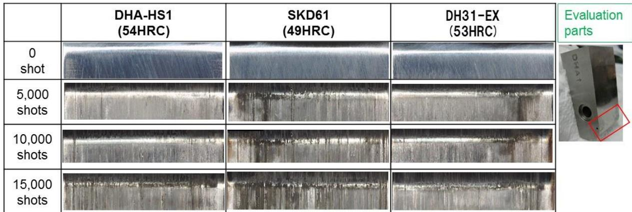
Fig. 7 Surface condition of upper evaluation parts after each shot.
