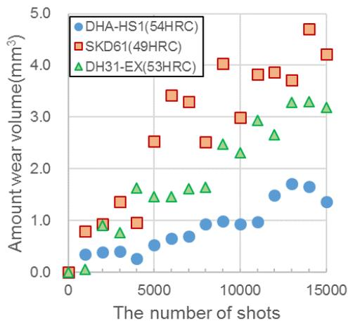
Fig. 8 Wear volume of upper evaluation parts after each shot.
