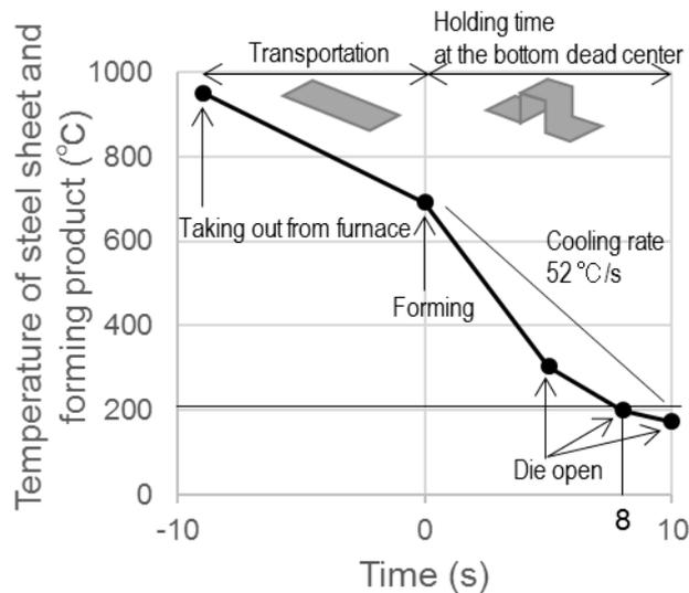
Fig. 3 Cooling curve of steel sheet.
