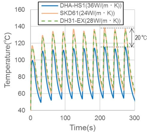
Fig. 10 Temperature of evaluation parts at 2 mm depth from the surface.
