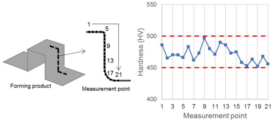
Fig. 4 Cross-section hardness of forming product.
