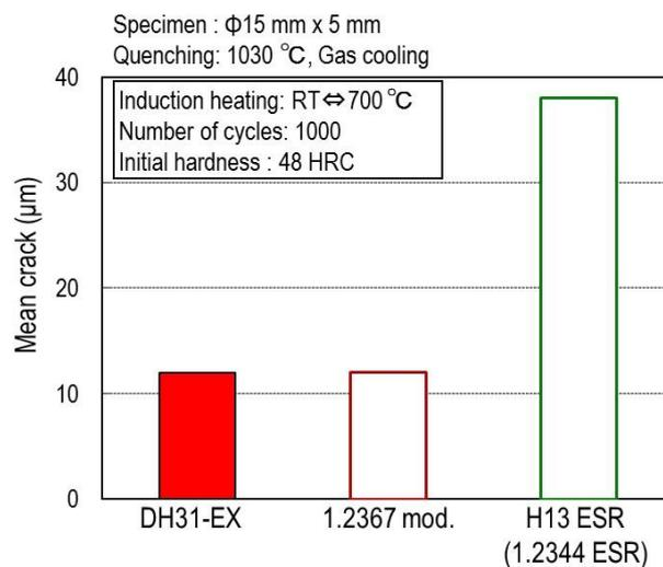
Fig. 5. Results of heat checking test
