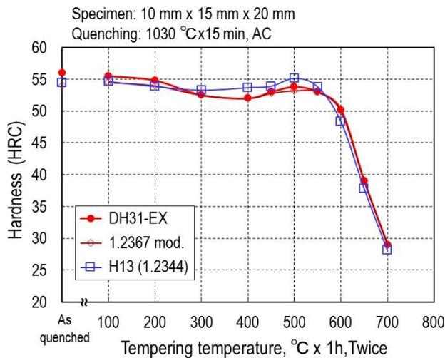
Fig. 8. Tempering temperature and hardness
