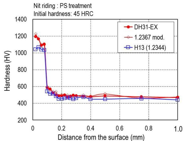
Fig. 9. Hardness distribution after nitriding
