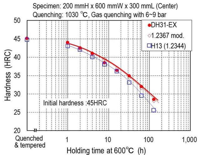
Fig. 7. Softening resistance at 600°C
