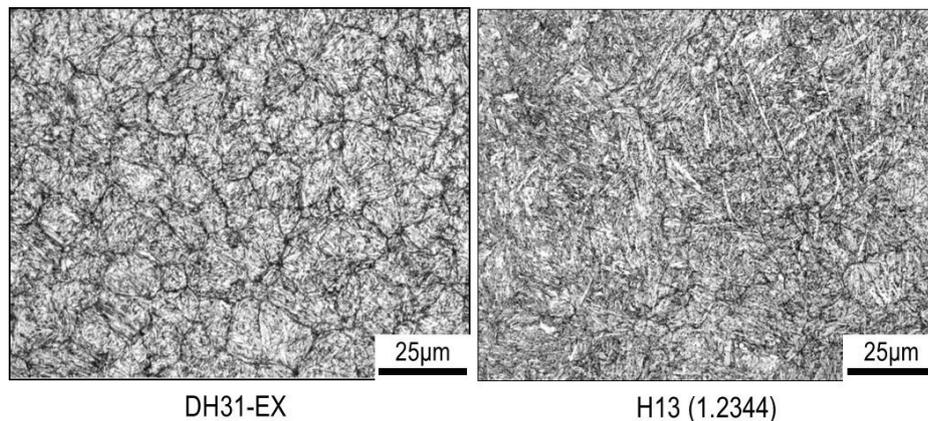
Photo. 2. Microstructure of center of heat-treated specimen simulating large molds
