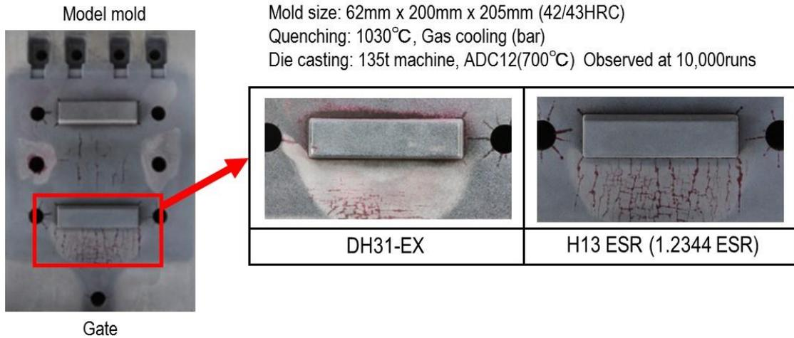
Photo. 3. Heat checking status by die casting trial
