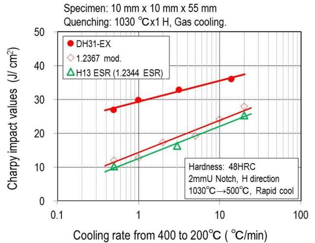
Fig. 4. Cooling rate dependency on impact values
