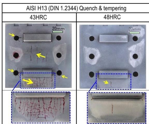
Photo. 1. Effect of hardness on heat checking
