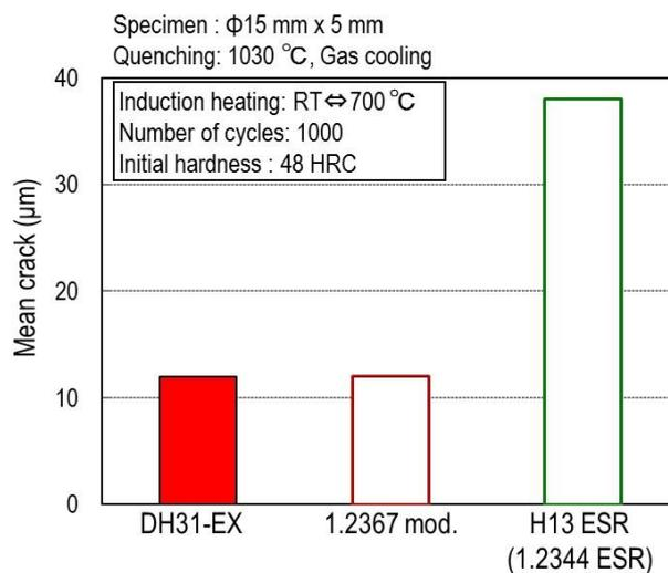
Fig. 5. Results of heat checking test
