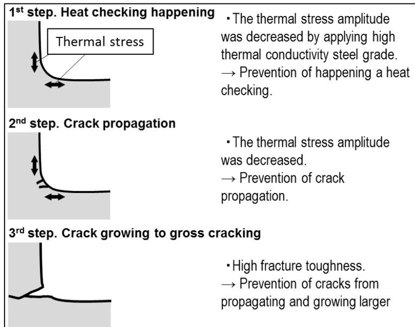
Figure 4 Schematic diagram of the gross crack mechanism.
