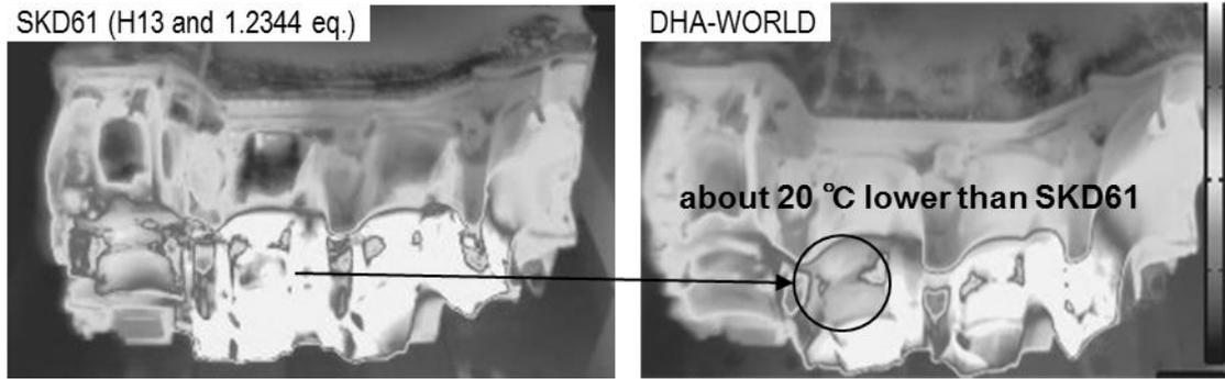
Figure 3 Comparison of the temperature profiles on the upper slide cores at 2 minutes after die opening.
