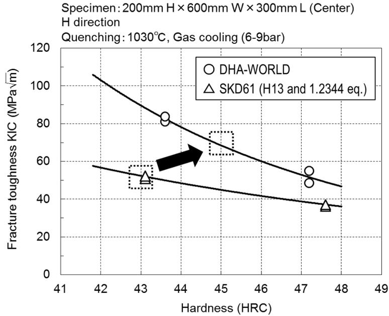
Figure 5 Fracture toughness
