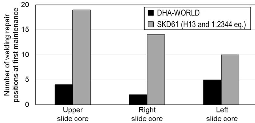
Figure 1 Number of welding repair positions at the first maintenance.
