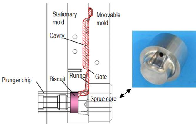
Figure 5 Application of DHA-THERMO in die casting test.
