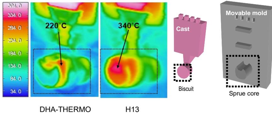
Figure 6 Surface temperature of sprue core.
