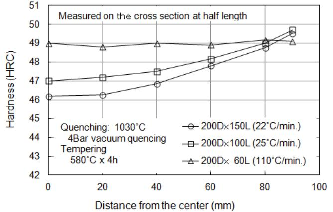
Figure 4 Examples of hardness in round bars 4Bar gas Quenched and tempered.
