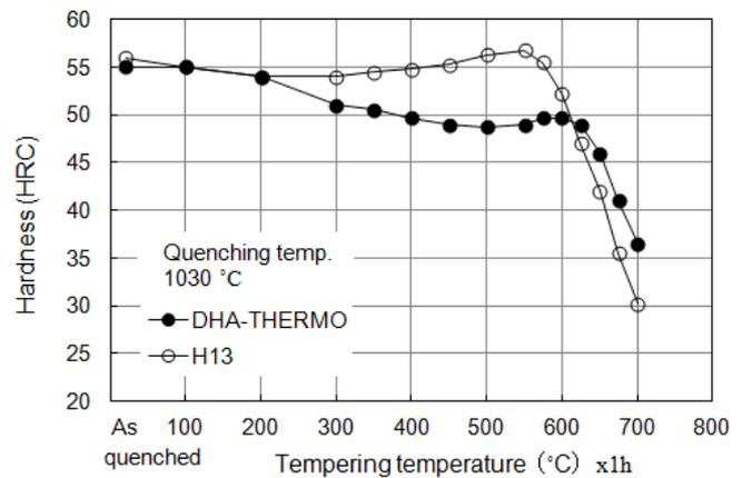
Figure 2 Hardness vs. tempering temperature.
