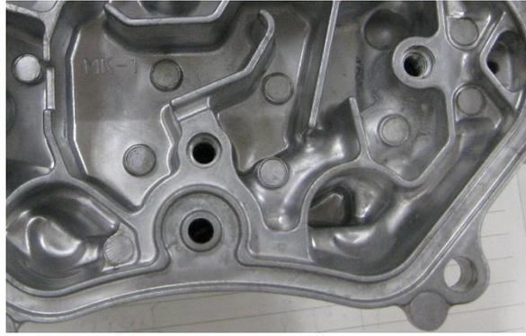
Figure 9 A part of Al die cast product where internal soundness was improved by the application of DHA-THERMO core pins.
