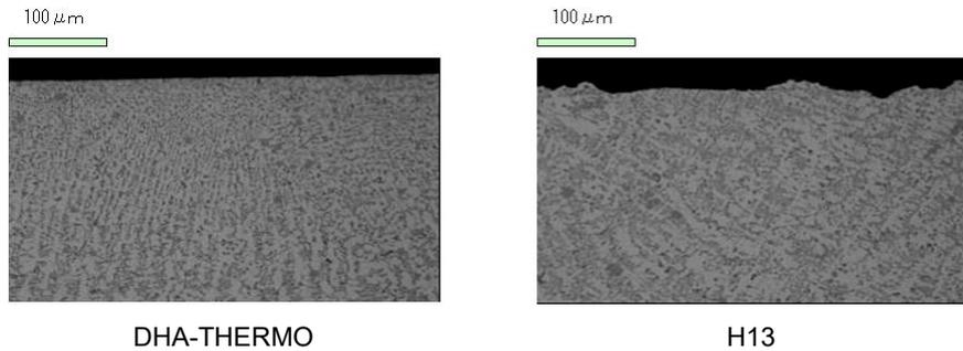
Figure 7 Optical micrographs taken from biscuit surface.
