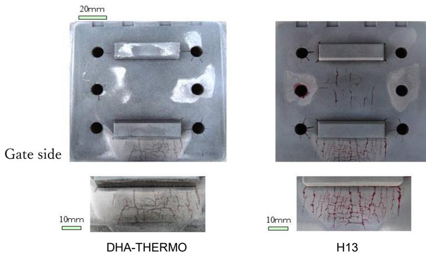
Figure 8 Heat checking observed on the surface of movable molds as of 10,000 shots.
