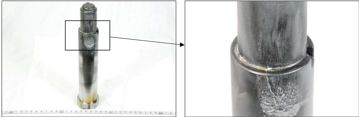
Figure 10 An example of core pin and failed area.
