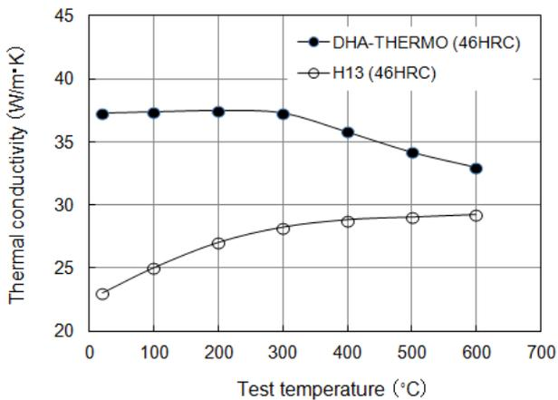
Figure 1 Thermal conductivity vs. test temperature.
