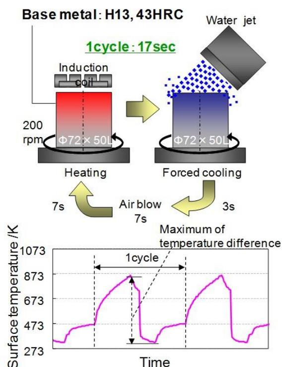
Fig. 7 Heat checking test procedures.
