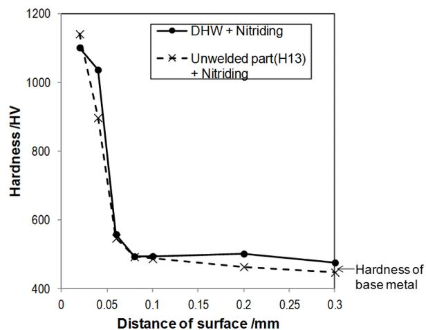
Fig.11 Hardness distribution after nitriding.
