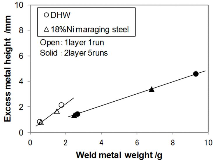
Fig. 12 Relationship between excess metal height and weld metal weight.
