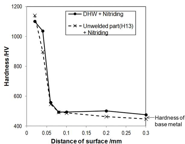
Fig.11 Hardness distribution after nitriding.
