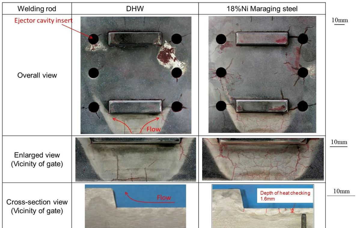
Fig. 9 Heat checking test result by actual die casting machine.
