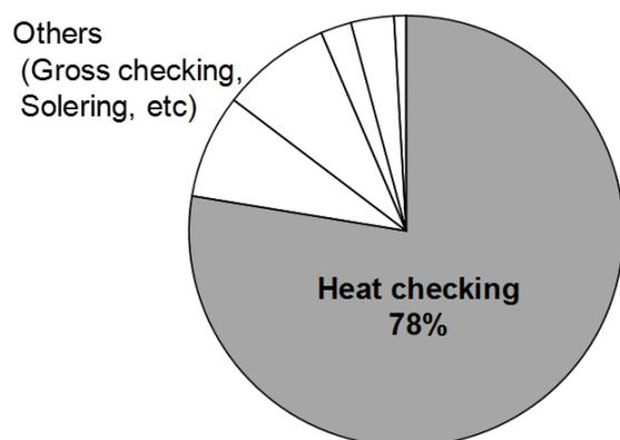
Fig. 1 Failure modes in die casting molds.
