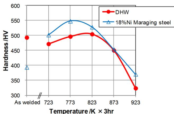
Fig. 10 Hardness with post-heating.
