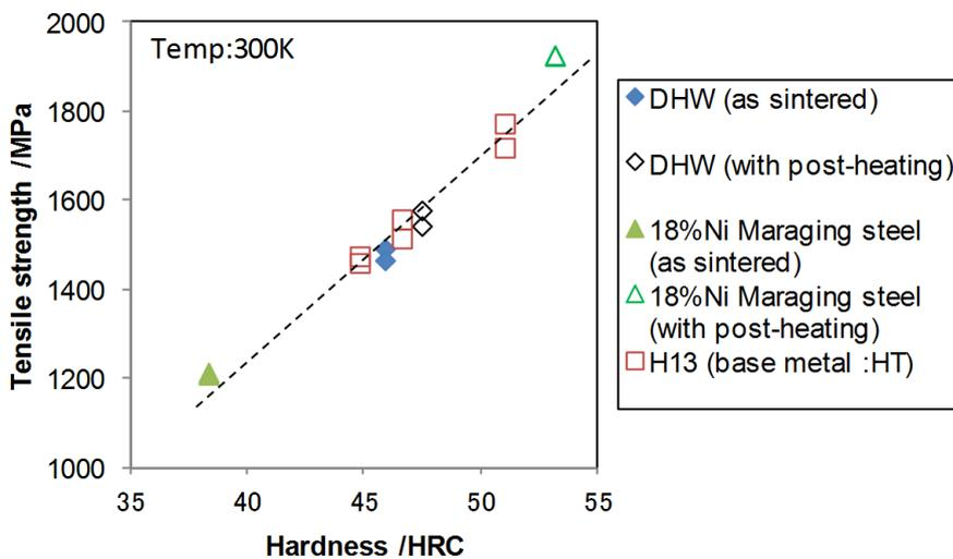
Fig. 19 Tensile strength at room temperature.
