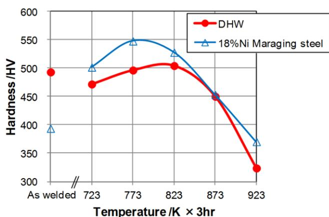
Fig. 10 Hardness with post-heating.
