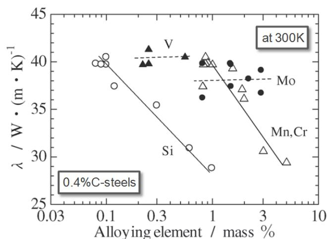
Fig. 2 Effects of alloying elements on thermal conductivity (46 HRC).
