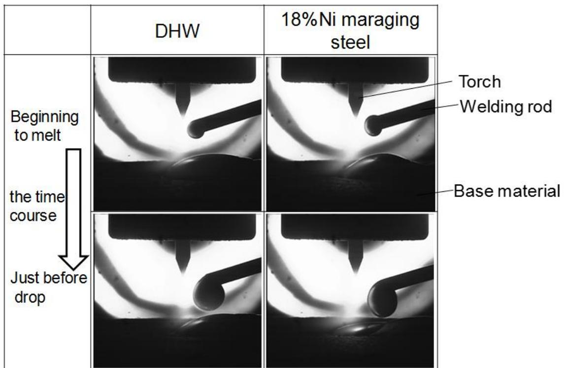
Fig. 13 An example of shots showing the behavior of droplets.
