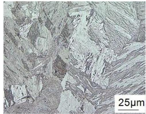
Fig. 5 Optical micrograph of welded DHW.
