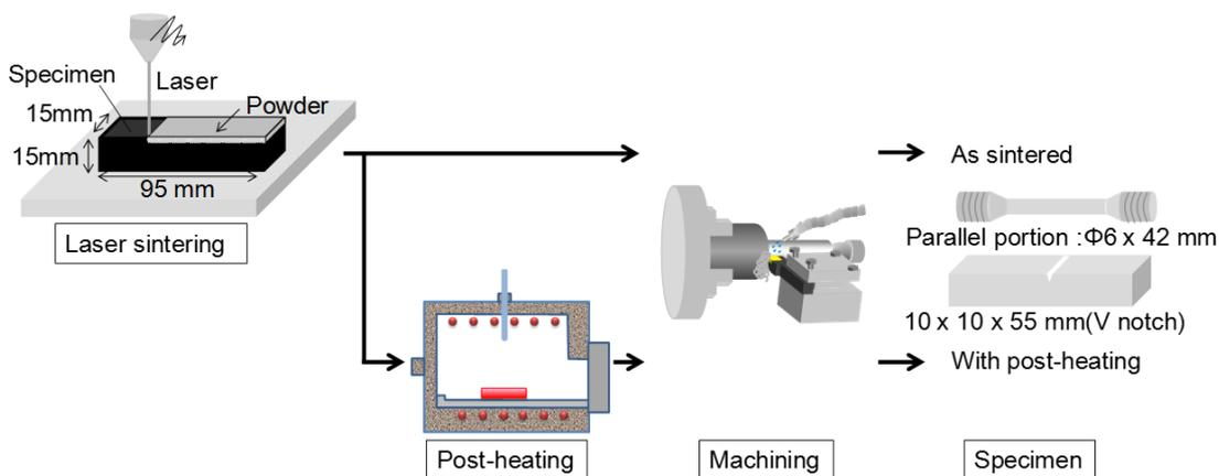
Fig. 17 Sampling procedures of tensile specimens.
