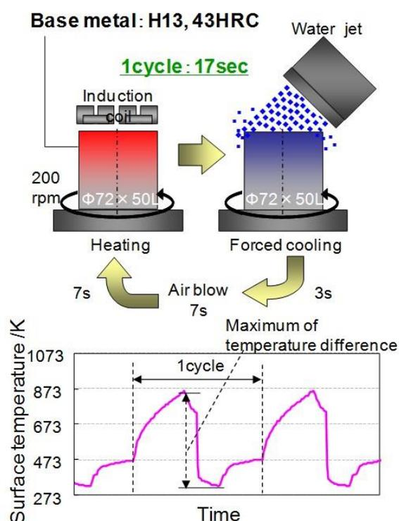
Fig. 7 Heat checking test procedures.
