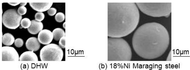
Fig. 16 SEM observation of powders used for laser sintering.
