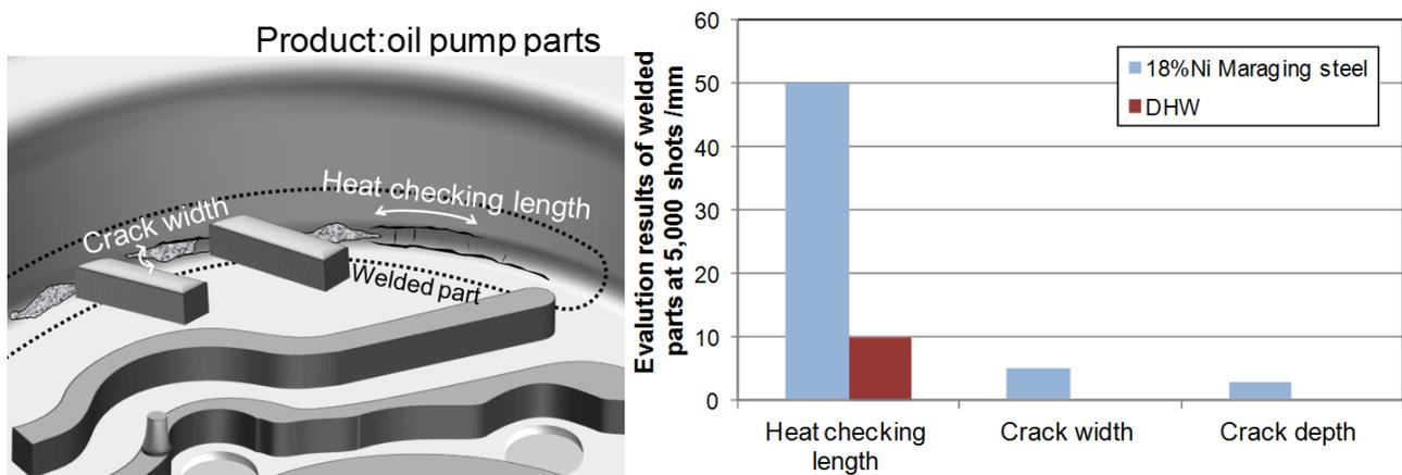
Fig. 14 An example of the application of DHW: Superior heat checking resistance.
