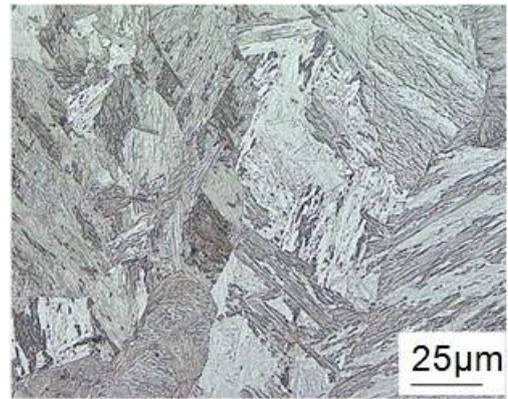
Fig. 5 Optical micrograph of welded DHW.
