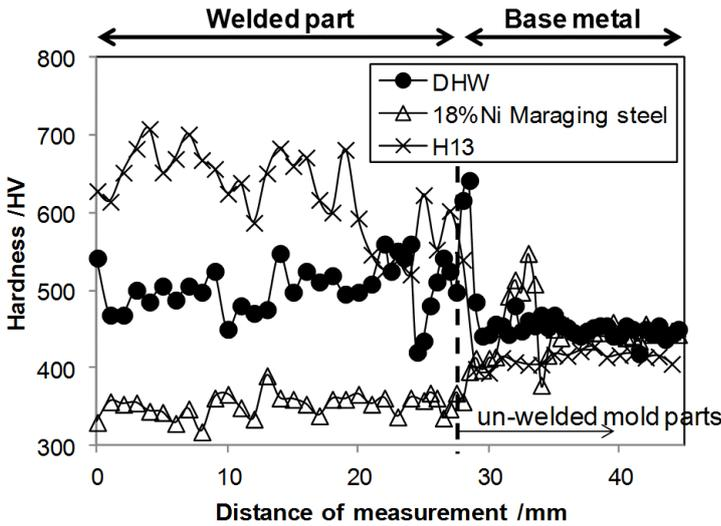
Fig. 4 Hardness distribution as welded.
