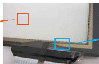
Blackening layer for metal-mesh electrode (STARMESH®-β1)
