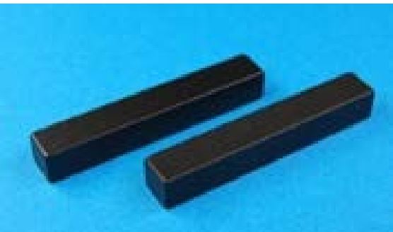
Heavy rare earth-free magnets by hot working process (in sheet form)
